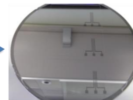
Master fabrication with negative photoresist SU8-50
